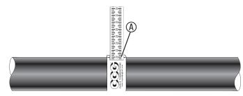
1. For accurate sizing, use a CCG Dimension Tape (4) on the outer cable sheath.
