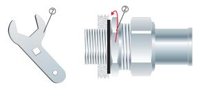
3. Screw the gland unit into the apparatus and tighten the inner ② to the installation torque using a CCG Spanner ⑧.
