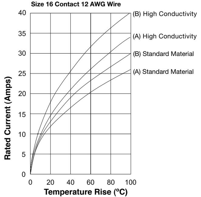
Above curves developed separately using Size 16 contact with 12 AWG wire. (A) Twelve (12) Size 16 contacts under load. (B) Six (6) Size 16 contacts under load.
