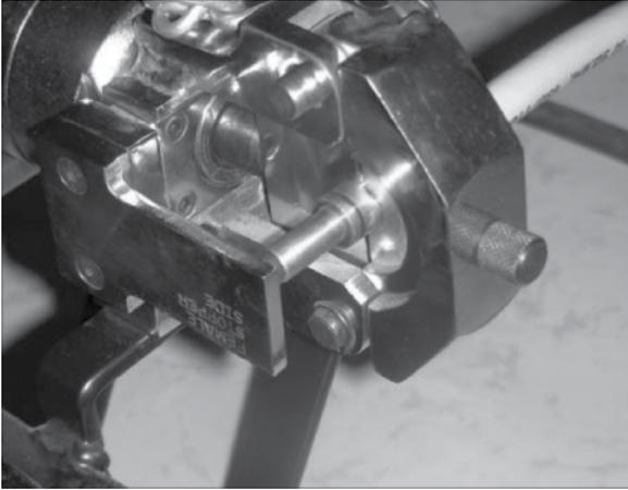
Same crimping tool (9504 -21 -0) is used for crimping '0' AWG wire and '4' AWG wire
