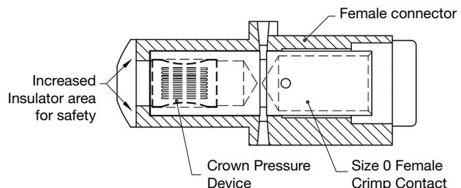
The connector was designed to pass the IEC 60950 (figure 2C) test probe which provides protection from electric shock and energy hazards.
