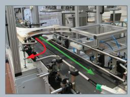
Located at the end of the machine, a pneumatic ejector allows to reject automatically the faulty cans
