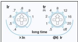
Long time delay setting knob is currently positioned at 0.8. If In is equaled to 1000A······
