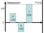
It is not common, but when the phase power is like the diagram, the synthetic power is 200.
