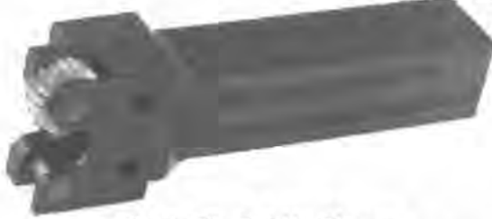
Single Die Set Up Shown (preferred method for "Straight" Knurling)
