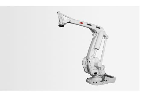
Thanks to its state-of-the-art 4-axes design, customers can look forward to a speedy machine that combines a 3.15 meter reach with a 250 kg payload, making it ideal for palletizing bags, boxes, crates, bottles and more. ABB reinforces its position as the global supplier of complete robot packaging line automation.
