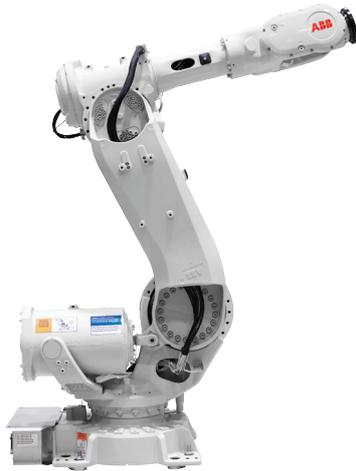
IRB 6640 Foundry Prime robot is designed for washing and cleaning applications. It is based on proven components from earlier generations, to ensure ease of maintenance and exchangeability as well as high up time.
