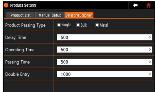
**i** This machine can set different delay time, the operating time for each output port. Refer to [4.7] for detail explains. This page does not consider delay/ operation time for output signal.
