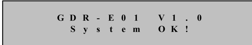
If there is a fault in the equipment, System Error! is displayed instead of System OK!
