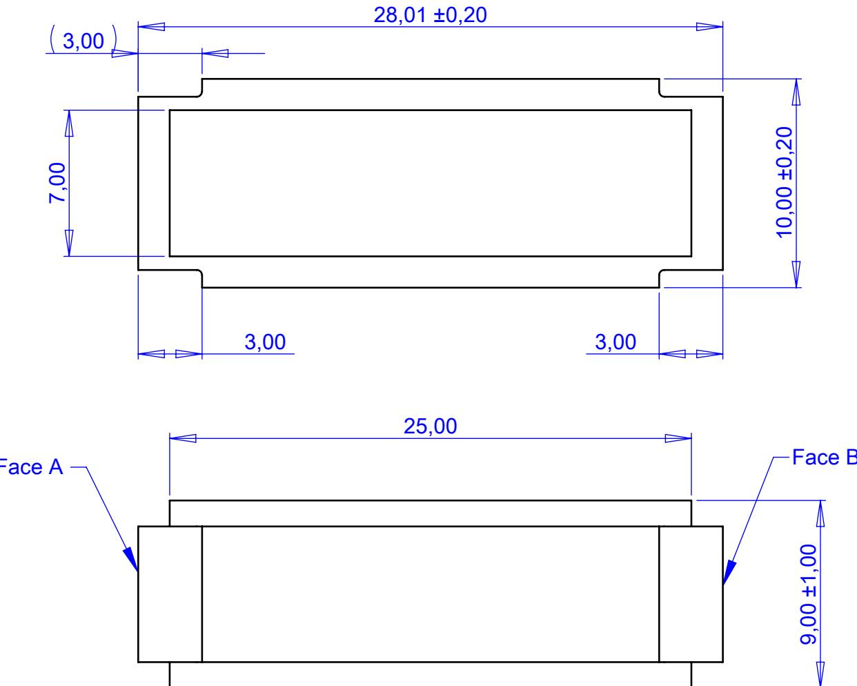
Dimensions and position of the M2,5 thread hole is valuable for face A and B
