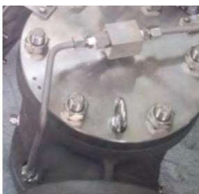
A backflow preventing device can be used to keep this situation in check. A sensing line is connected to the exit side of the main body and the main dome, preventing backflow and guaranteeing an accurate pressure differential.
