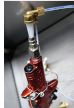
Plastic Plug inserted into the air passage way of the spray gun
