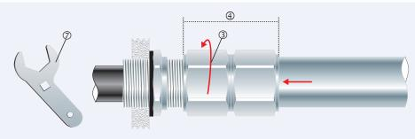
Pass the cable end through the conduit assembly ④ and the gland assembly. Tighten the outer ③ to the installation torque using a CCG Spanner ⑦ to produce a seal and grip on the cable.
