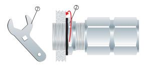
Screw the gland unit into the apparatus. Tighten the inner until hand tight ② using a CCG Spanner 7 with 1/4 turn.
