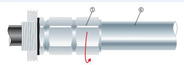
5. Fit the threaded conduit end 6 into the female rotating threads 5 as indicated.
