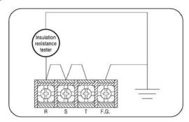
Operate the test by short-circuiting the power terminal as shown in above picture. Do not operate the Insulation Resistance Test to the control terminal. Use 500V Insulation resistance tester.
