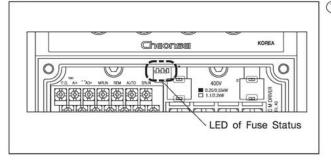
① If the front terminal cover of Driver is opened, three Red LEDs are in the position as shown in the left picture. It shows the fuse status for R, S, T phase from the left side and, if fuse is normal status, the LEDs light up when power is turned on.
