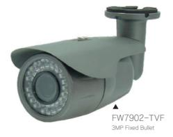
**FW7902-TVF** is a high quality Bullet type IP camera which is equipped with 3.21MP(effective pixel) Progressive Scan CMOS image Sensor. With the highest sensitivity Starvis sensor, It is especially superior in low light condition. As it supports simultaneous H.265, H.264 and MJPEG Video Compression, less network bandwidth and storage space required. It also delivers high quality video image at 30fps@3M(2048x1536) in progressive mode.
