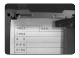
By side: Insert the paper from left to right then wait for it to work automatically. From the picture above, the paper should be inserted right till the end.
