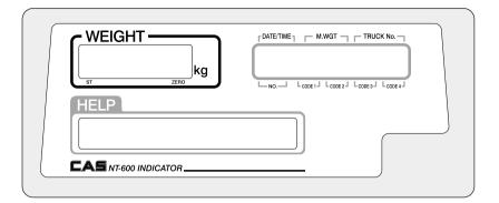
ST Lamp : Lights on when weight is stable ZERO Lamp : Lights on when weight is 0 kg DATE/TIME : Current Date or Time is displayed.
