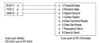
COM 1 : Secondary Display (CD Series) Connector specification Connecting with Secondary display
