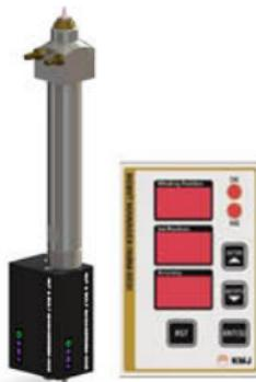
It is a device which detects the defects in nut and bolt such as nut projection defect, bolt length defect, installed reverse nut, no nut, eccentricity due to fallen nut or welding defect caused by application of non-electricity and it stops welding operation to prevent welding defect, and after welding it discriminates whether the welding is normal and indicates the result to the operator.
