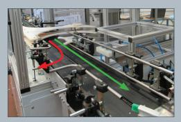
Located at the end of the machine, a pneumatic ejector allows to reject automatically the faulty cans
