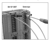
In case of SM-S7-300T, just insert in the left arrow direction to complete wiring, but screw type is wired using a tool as shown in the right arrow, so the workability of SM-S7-300T is much better.
