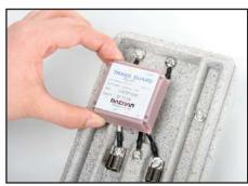
Mount the protective module into the space above transformer. Be sure to insert each U-wire connector to appropriate place where screw bolt is already loosen.
