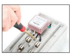
Tighten all 5 screw bolts. Make sure U-wire connectors are does not slip out from the screw bolts.
