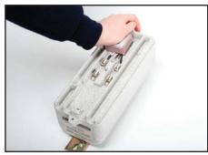
Press down the module toward the body of neon transformer in order to minimize gap between the module and transformer. Cover lid of neon transformer will not be closed if not pressed down correctly.
