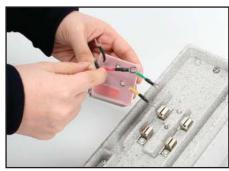
Prepare the protection module by pulling out lead wires outward
