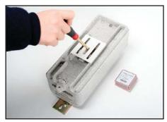
Use screw driver to unscrew the protective lid of primary input
