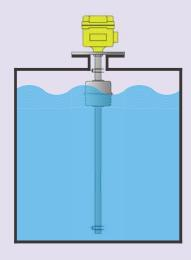
When the liquid level goes Up to reach the HIGH/A point, the HIGH/A indcator turns on. At the same time, the HIGH/A contact signal activates the connected buzzer and purmp.
