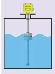
When the liquid level goes Up to reach the START point, the START indicator turns on. At the same time, the START contact signal activates the connected pump.
