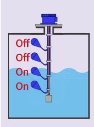
When the liquid level goes Up to reach the POINT2 point, the Point2 indcator turns on. At the same time, the Point1 contact signal activates the connected pump. When the liquid level goes Down to reach the POINT2 point, the Point2 indcator turns off. At the same time, the Point2 contact signal is not out and
