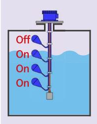
When the liquid level goes Up to reach the POINT3 point, the Point3 indcator turns on. At the same time, the Point3 contact signal activates the connected pump. When the liquid level goes Down to reach the POINT3 point, the Point3 indcator turns off. At the same time, the Point3 contact signal is not out and
