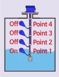
When the liquid level goes Up to reach the POINT1 point, the Point1 indcator turns on. At the same time, the Point1 contact signal activates the connected pump. When the liquid level goes Down to reach the POINT1 point, the Point1 indcator turns off. At the same time, the Point1 contact signal is not out and
