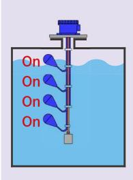
When the liquid level goes Up to reach the POINT4 point, the Point4 indcator turns on. At the same time, the Point4 contact signal activates the connected pump. When the liquid level goes Down to reach the POINT4 point, the Point4 indcator turns off. At the same time, the Point4 contact signal is not out and
