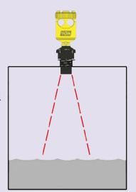
\* Water drops on the top of the tank can cause sensor malfunction.
