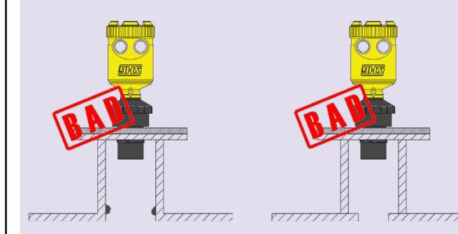
If there is a buy or a welding seam in the inner wall surface of the nozzle it can be recognized in detection target. After installation, you must remove.
