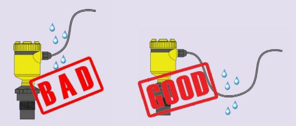
As shown in the above pictures, slacken the cable to the bottom in order to prevent water (rain, any liquid) coming in through the cable gland.
