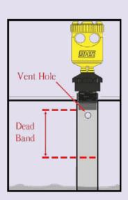
If there are water drops on the top of the tank, be cautious not to affect the sensor beaming. Swell due to water drops can occur sensor malfunction.
