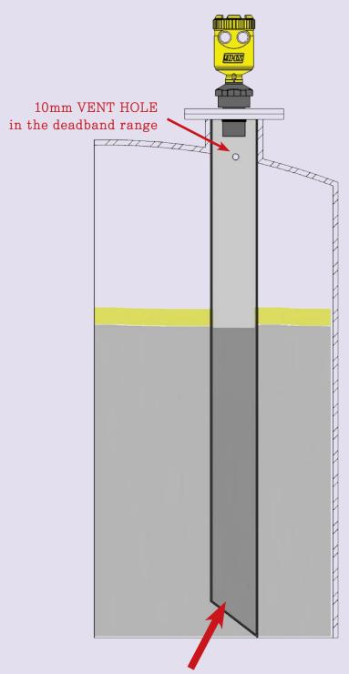
So as to cut into the bottom 15  $\sim$  45  $^{^{\circ}}$  float in the pipe it is not flowing net installed.
