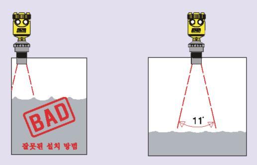
Beamwidth is about 11. Considering this beamwidth, install the sensor securing enough distance from the wall.
