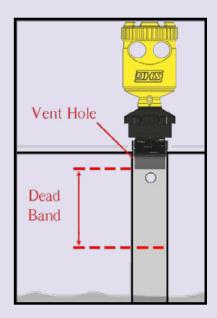
You can prevent malfunction with protection pipe when suspended solid exist in the tank as shwon in the above pictures.
