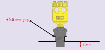
\* The floor surface sensor must be installed at least 30mm to enter the inner tank...
