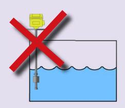
Install the sensor so that it is perpendicular.
