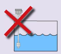
Install the sensor so that it is perpendicular. Float of the sensor does not touch the wall of the tank.
