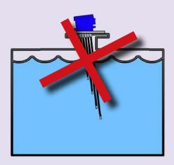
Install the sensor so that it is perpendicular.
