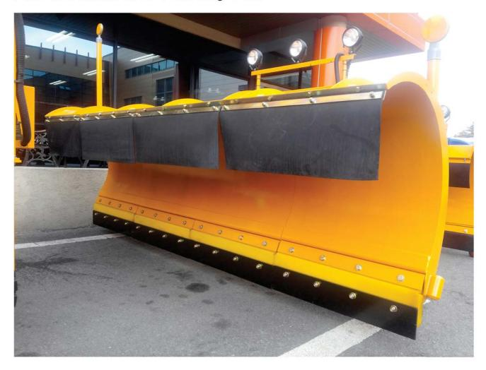
Steel sheet of snow removing shovel blade is hard and sharp making it damage roads and structures. It is relatively vulnerable to abrasion and more expensive compared to rubber products. Rubber shovel blade is a product that places rubber shovel blade on the bottom part of shovel blade improving its safety and durability while reducing maintenance cost.
