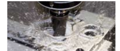
Machining details Holediameter: D40 mm Material: Carbon steel
