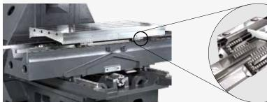
Grease lubrication for all axes is a standard feature.
