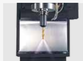
Through-spindle coolant spray system
