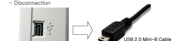
Exit the application provided to user PC, and then remove the cable from the USB terminal of the main body.
