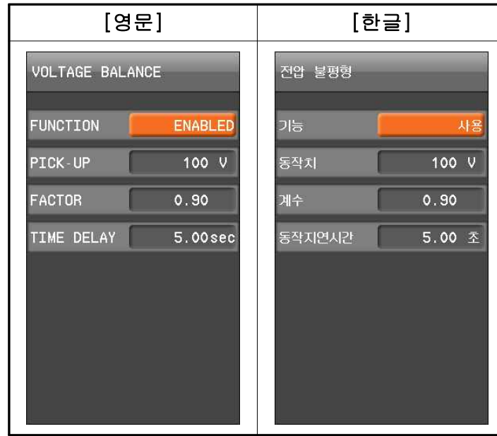
&lt;Figure. VOLTAGE BALANCE 설정 화면&gt;
