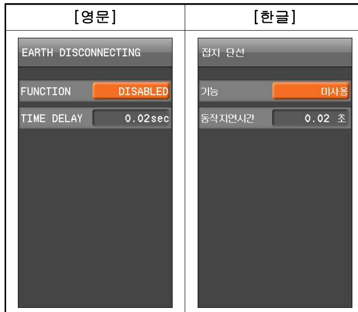
<Figure. EARTH DISCONNECTING 설정 화면>
