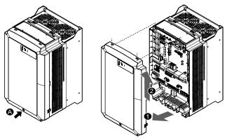
2 Refer to the following figure to replace the four M3 screws on the inverter's control board with the four M3 x 18 brass studs.
