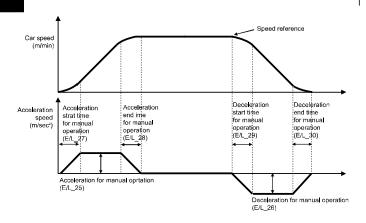
E/L\_26, E/L\_29, and E/L\_30 define the deceleration conditions to perform an S-curve deceleration for maintaining comfortability of the ride when a deceleration results from the change of multifunction inputs for manual operation to a different speed reference (for example, 15 m/m  $\rightarrow$  3 m/m).
