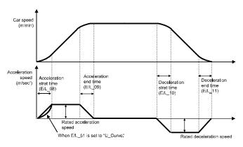
As shown in the figure above, linear acceleration (solid line) is made when E/L\_51 is set to "Linear", and curved acceleration (dotted line) is made when E/L\_51 is set to "U-curve". The setting at E/L\_51 is applied only to the starting section of the acceleration, and a linear acceleration will be made for the remaining section regardless of the setting at E/L\_51.
