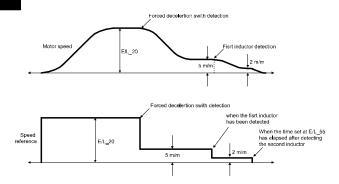
To precisely stop the car at the floor height level during base floor or nearest floor operation, appropriately adjust the setting at  $E/L_55$ , which is the delay time until the speed reference becomes "o" after the car meets two inductors. Be careful not to set the time at  $E/L_55$  too long because it may cause the car to miss the floor height level.
