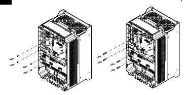
Properly install the ELIO add-on module after aligning its connectors to those on the inverter's control board, then secure it to the brass studs by installing the four M<sub>3</sub> x 8 fix bolts (torque: 12 kgf-cm).
