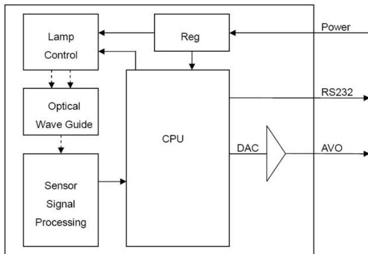
\* CO<sub>2</sub> 측정(ppm) = Output Voltage- 0.5/ (4.5 - 0.5) Voltage x F.S. ppm
