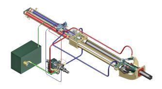
Direct connecting main pump and hydraulic cylinders improve pumping efficiency
