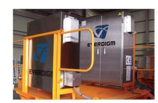
1 All cable connectors to controller placed inside the stainless cage provide complete protection for electronic system from water and dust.
