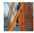
Once each ballast block is just simply inserted in the compartment in sequence, then they are self-positioned and automatically aligned in place, thanks to special-designed compartment. Zero space and tight-contact between counter-weight blocks.
