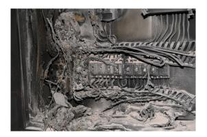
▲ fire of switchboard \_ TS-60 minimize the damage by early detecting of these fire.
