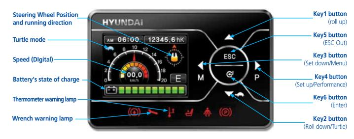
The LCD color monitor with 3.5 inch graphic smart display allows the operator to easily and efficiently control the machine. The monitor provides information about speed & accelerator level, steer angle & travel direction, battery discharge indicator, hour meter & working mode. The optional load indicator displays the load weight in the monitor. The operator can select various performance modes to meet all working conditions. It is available multi-languages (maximum 12) for operator.
