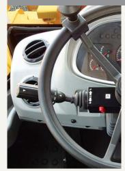
A single lever on the left side of the steering column gives the operator fast, easy control of speed and direction. Push the lever forward to go forward, pull it back for reverse. Travelling is automatically changed from 1st stage to given stage according to travel speed and tractive effort. The operator can select two kinds of automatic modes (1st  $\leftrightarrow$  4th).
