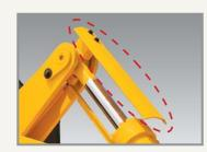
**Bucket cylinder guard** This guard helps to prevent possible damage from load material.
