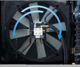
low noise is realized by applying hydraulic cooling fan that senses coolant temperature, intake air temperature, transmission oil temperature and hydraulic oil
