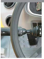
A single lever on the left side of the steering column gives the operator fast, easy control of speed and direction. Push the lever forward to go forward, pull it back for reverse. Travelling is automatically changed from 1st stage to given stage according to travel speed and tractive effort. The operator can select two kinds of automatic modes (1st  $\leftrightarrow$  4th, 2nd  $\leftrightarrow$  4th).
