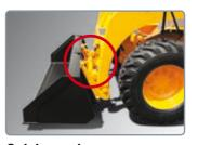
Quick attachment system Quick attachment device provides fast cycle time and easy operation.
