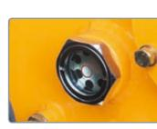
Tilting canopy for easy access Hydraulic oil level gauge
