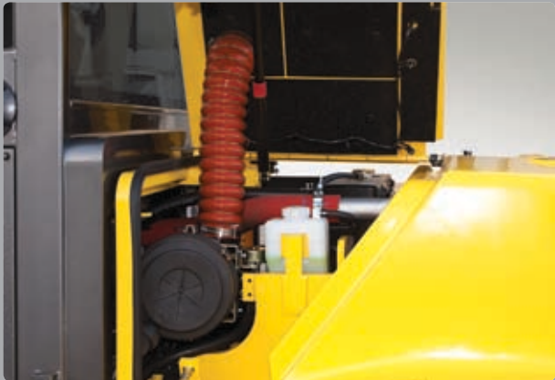
Easy change air cleaner The air filter is readily accessible for cleaning or replacement.
