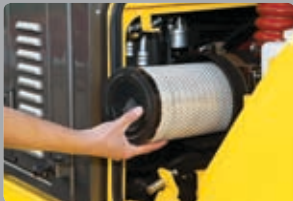
Easy change air cleaner The air filter is readily accessible for cleaning or replacement.
