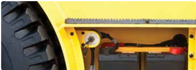
Master Switch A master switch disconnects the battery power to protect the electrical system from excess electrical drainage. (optional)
