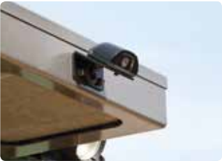
Rear View Camera (Option) The rear view camera makes the operation more easy and convenient. And the monitor supports 4 camera channels.
