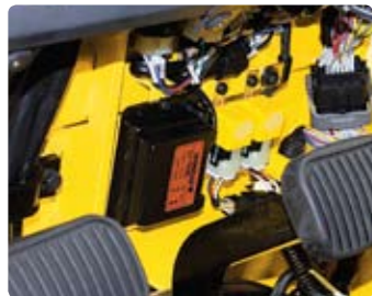
Improvement in Maintenance of Electric Parts Various electric parts are centralized in dash board resulting in effortless troubleshooting.
