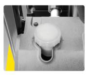
Brake Fluid Reservoir with Level Switch
