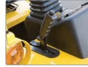
Integrated electrical devices enhanced Ratchet type parking brake requires less effort from the operator to set.
