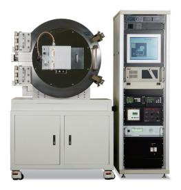
CARBOZEN™-C(PECVD: Plasma Enhanced CVD)SERIES is in the CVD method which uses plasma and it demands decompose ion gas, utilizing a generated glow discharge.
