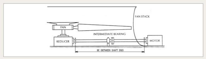
However, the long axis of the coupling made of the composite material which weighs only 20 % of the steel material can reduce deflection conspicuously compared to the same standard coupling made of the steel material. Once the composite material is used, the length of the axis can be extended by as much as 80% without using the fixture and bearings as shown in the piicture below.
