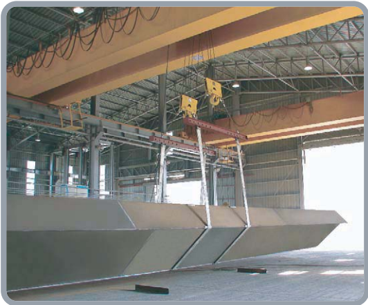
According as the target products, we supply the special hanging jig.
