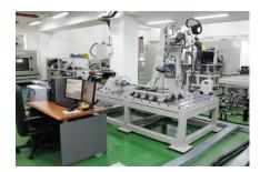
This system consists of a Servo system, which includes one channel hydraulic servo actuator, CAN network for EPS control, a fixture to fix C-EPS, torque cell fixture, and a base plate.
